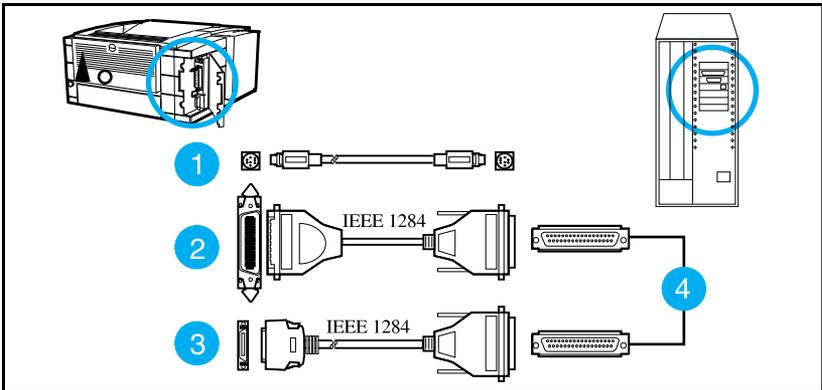
Figure 12 HP LaserJet 5P/5MP, 6P/6MP Printer Interface Connections
