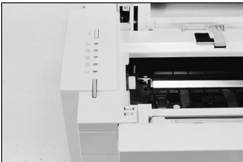
Figure 17 Left Side Cover Release Latch (5P/5MP shown)
