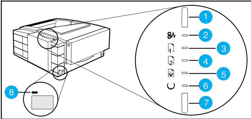
**Figure 5** 5P/5MP Status Panel Buttons and Lights
