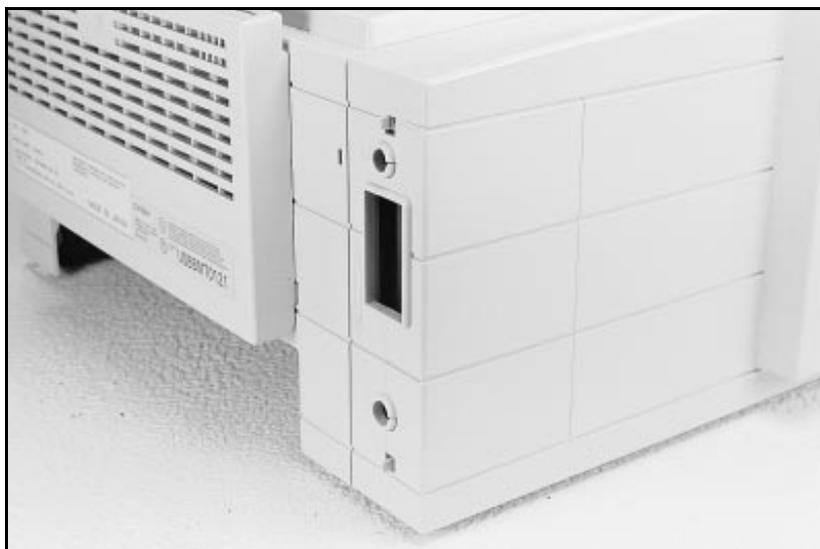
Figure 15 5P/5MP I/O Cover Release Tabs
