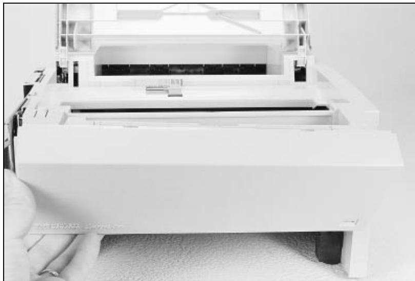
Figure 18 Removing Tray 1.
