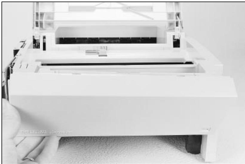
Figure 21 Removing Tray 1.
