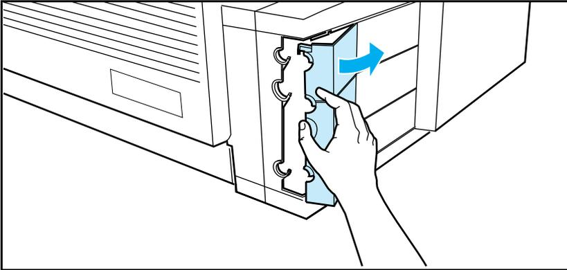
Figure -16 6P/6MP I/O Cover Finger Slot
