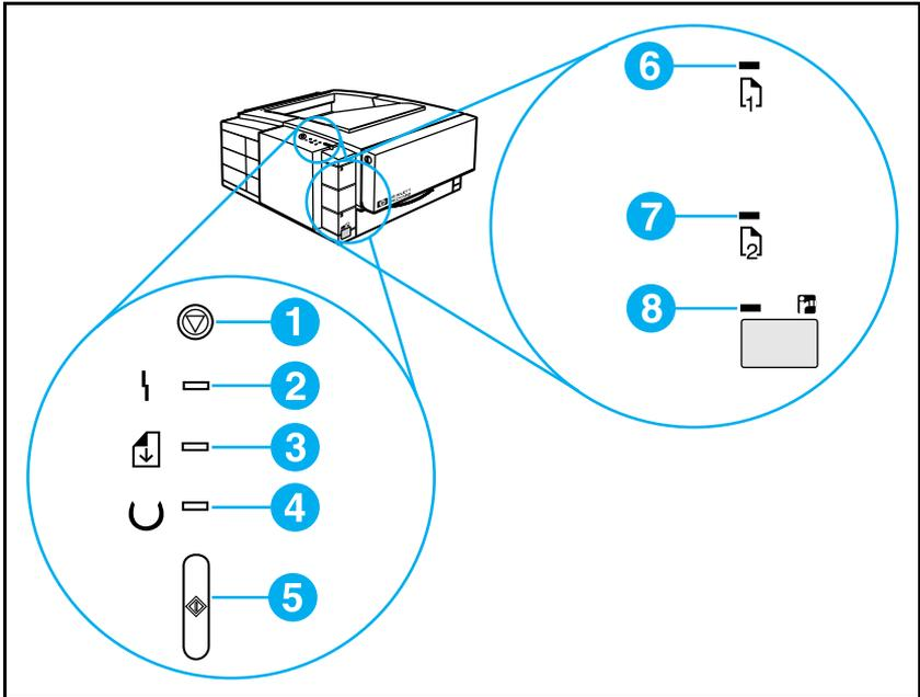
Figure 6 6P/6MP Status Panel Buttons and Lights
