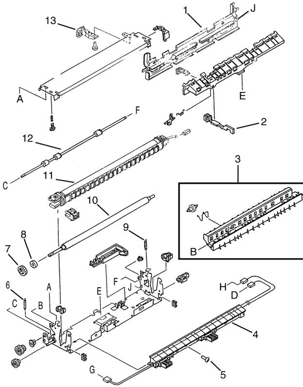
Figure 39. HP LaserJet 5P/6P Fusing Assembly
