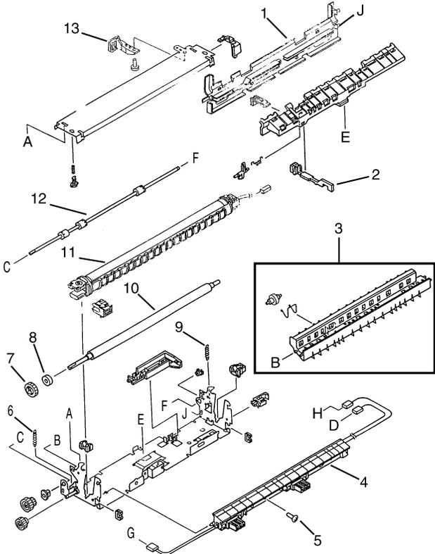
Figure 36. HP LaserJet 5P Fusing Assembly
