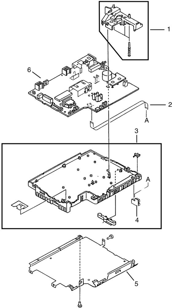
Figure 36. DC Controller Assembly
