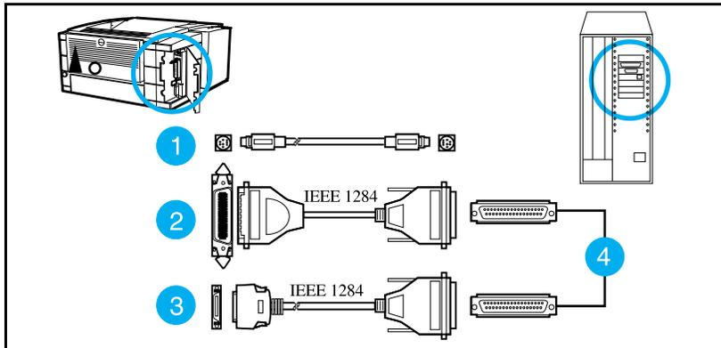
Figure 11 HP LaserJet 5P/5MP Printer Interface Connections
