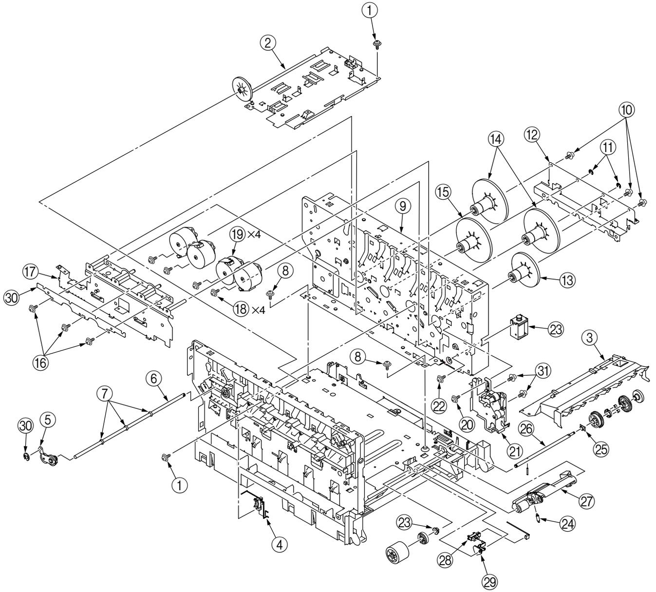
Figure 2-2-18 Main Motors / Solenoid / Paper-End Sensor
