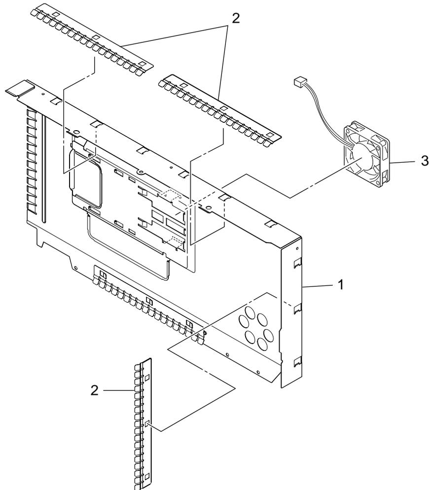
Figure 7-8-1 Plate\_Assy-Shield (C5300)
