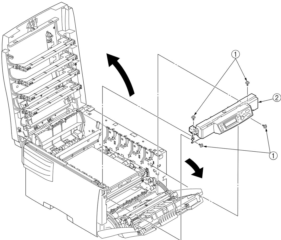
Figure 2-2-10 Control Panel Assy
