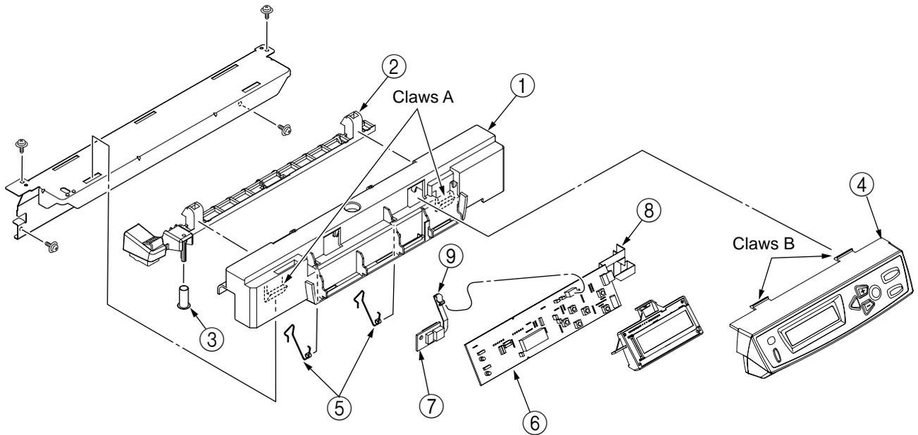
Figure 2-2-11 Board RSP / Environment Sensor / Top Cover Handle
