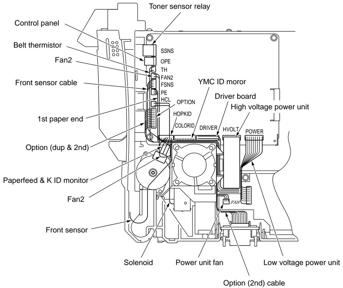
Figure 2-2-8-3 Print Engine Controller Board Cable Route
