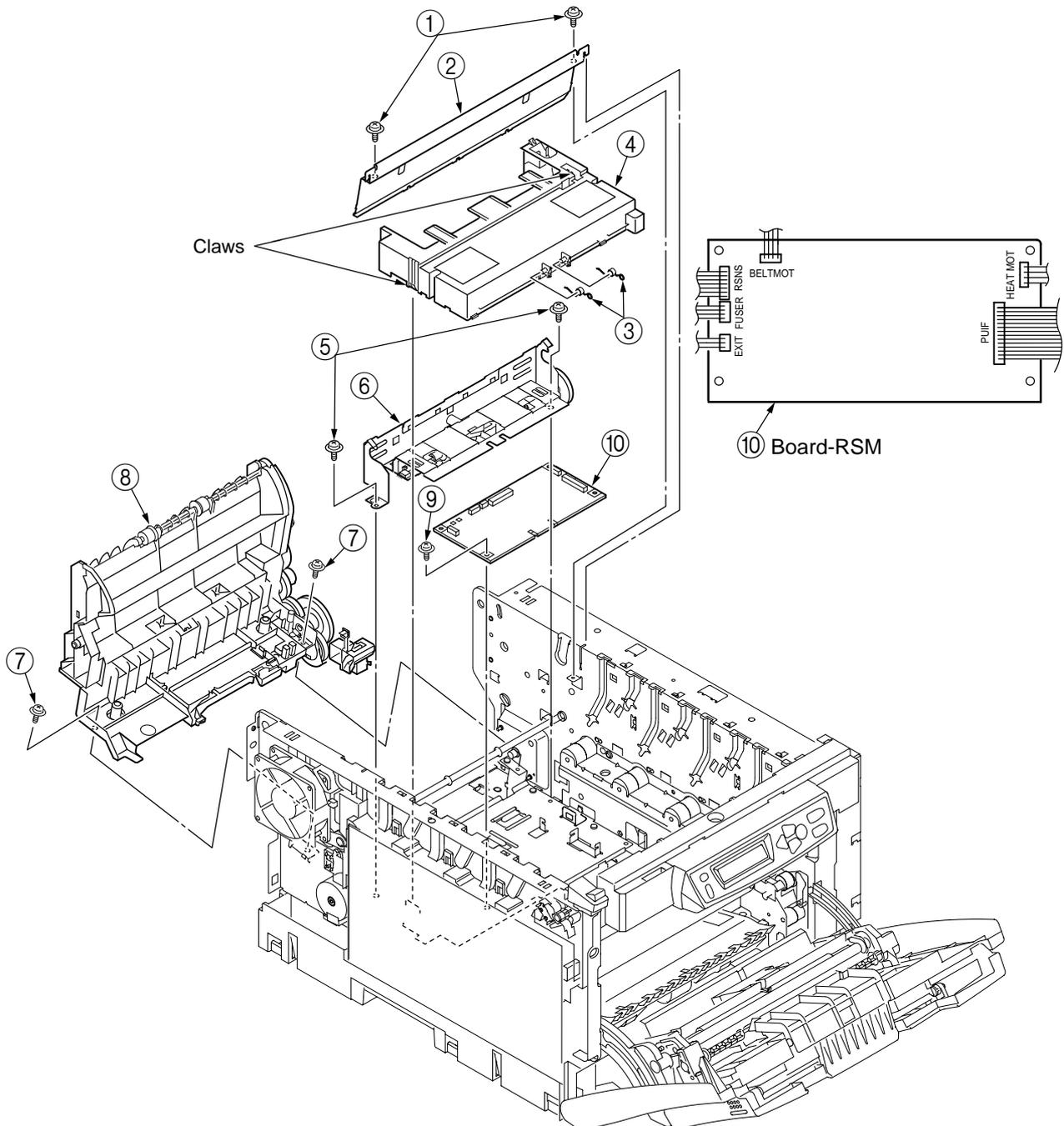
Figure 2-2-14-1 Guide - Eject Assy / Color Registration Assy / Board-RSM
