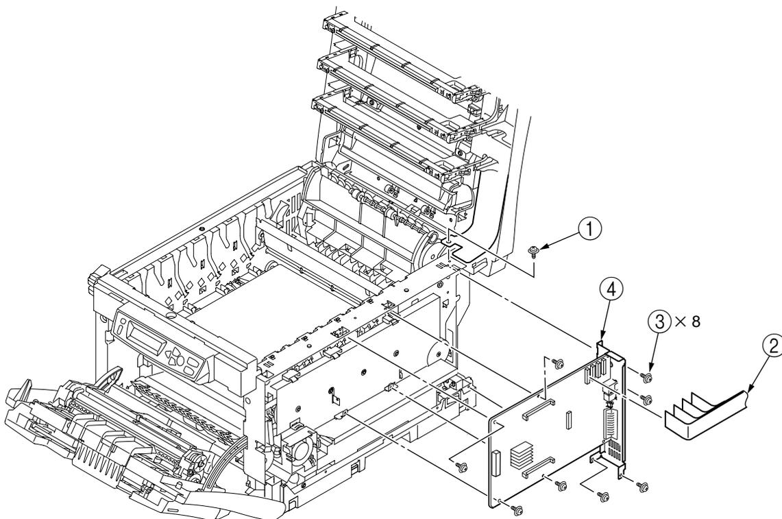
Figure 2-2-7-1 Controller PWB (C5300)
