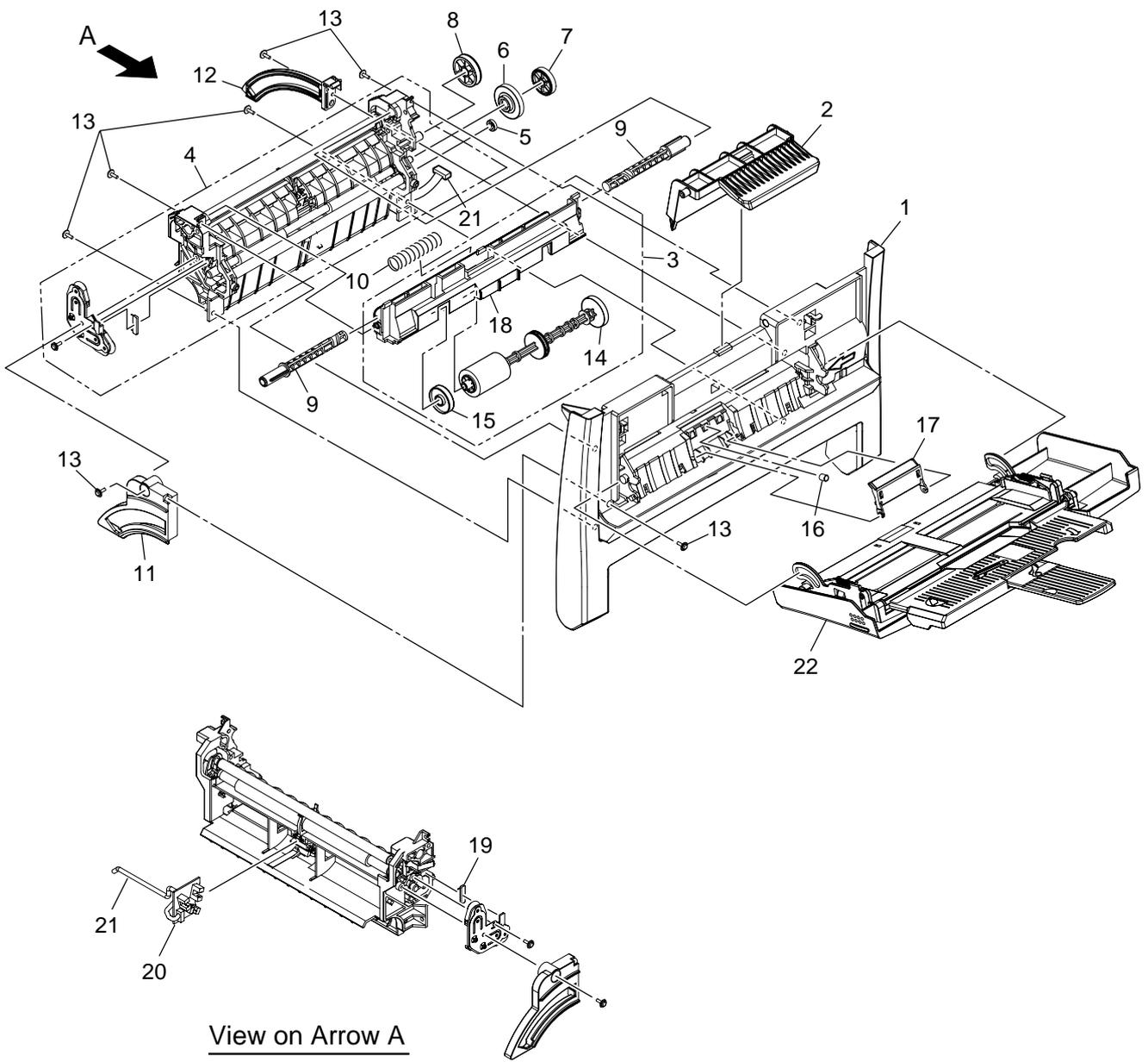
Figure 7-4 Feeder\_Unit
