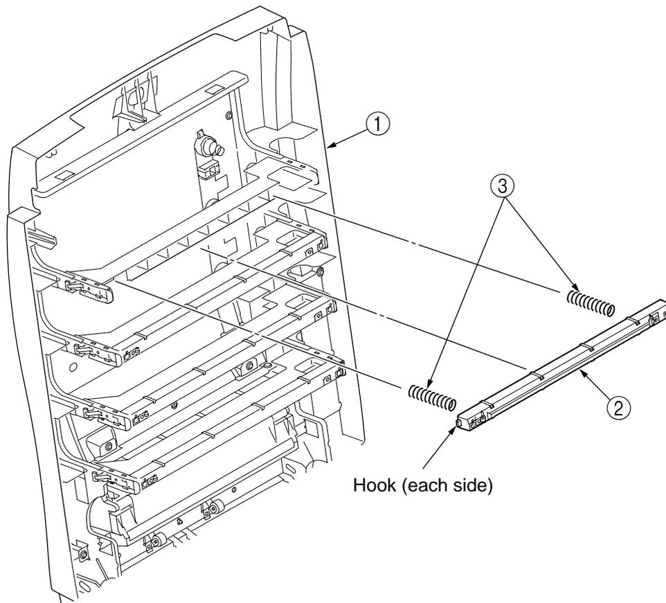
Figure 2-2-6 LED Assy / LED Assy Springs
