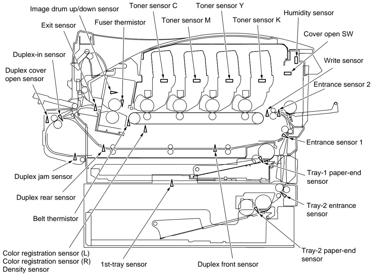
Figure 3-1 Switch Sensor Positions
