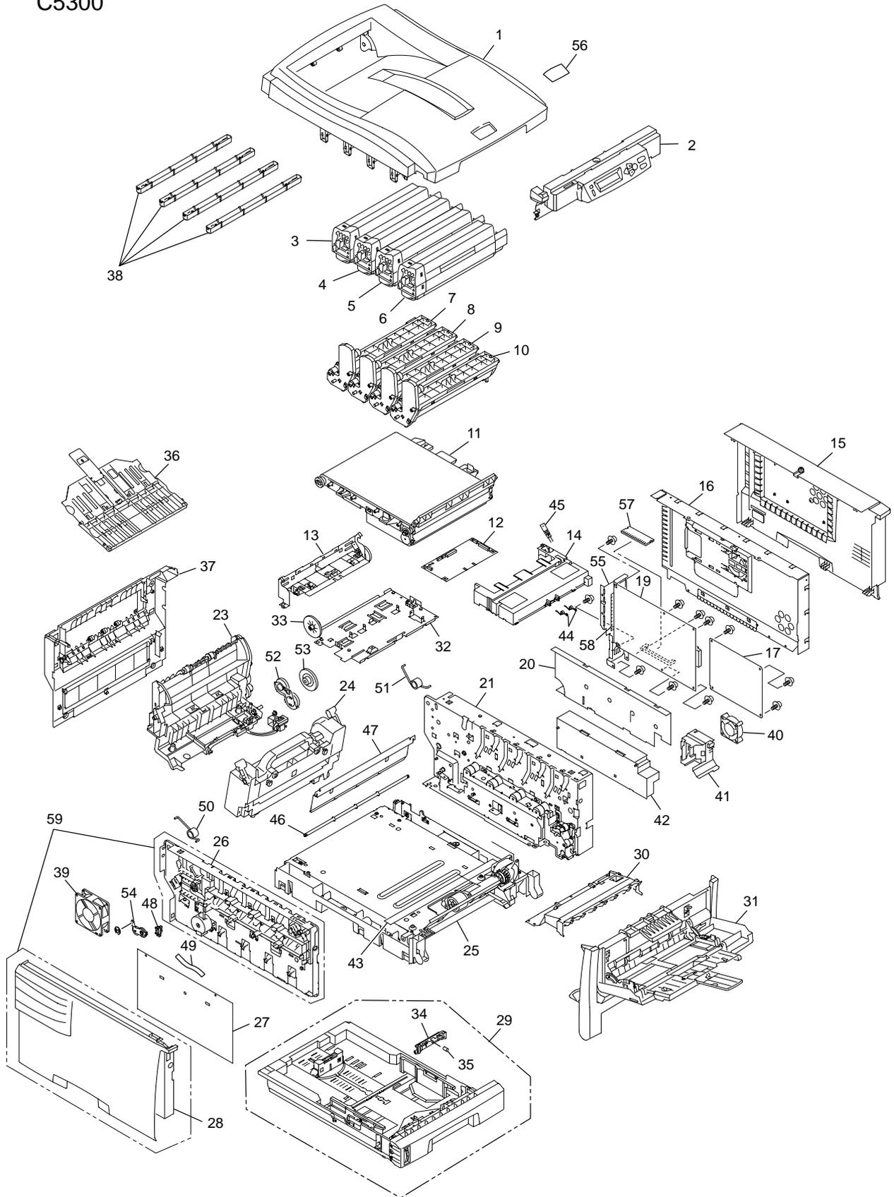
Figure 7-1-1 Parts Layout (C5300)
