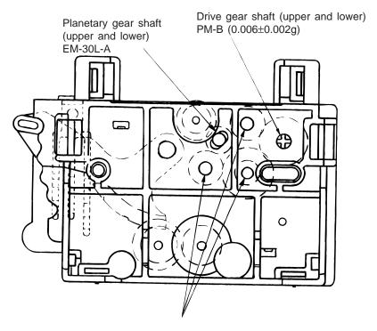
Idle gear shaft (upper and lower) PM-B (0.006±0.002g)
