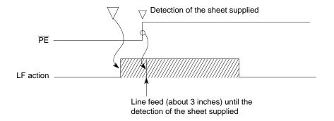
When the "FF/LOAD" button is pressed, the LF motor feeds in the sheet about 3 inches. When the LF motor completes its operation and the sheet has not been fed in, an alarm condition results.
