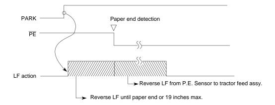
The alarm LED lights up when paper end is not detected after 19 inches of reverse feeding.
