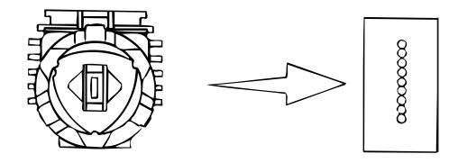
Figure 2-2 Arrangement of the head pins
