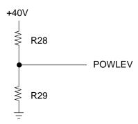
The head drive time is lengthened to compensate for the amount of voltage drop by monitoring the POWLEV signal once every 500  $\mu$  sec. to control and maintain the impact necessary for each printing pin at the fixed value.
