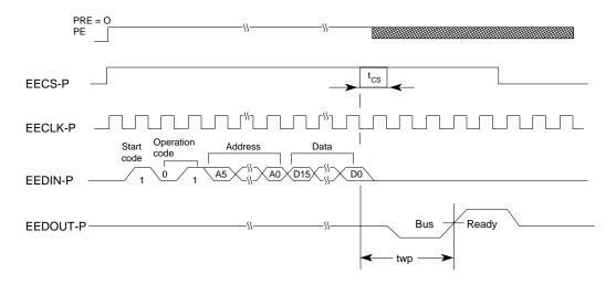
Write cycle timing (WRITE)
