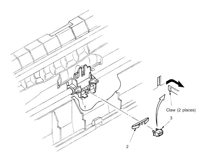
**Note:** Small round hole with metal tip on back of roller holder assy 3 should be facing up when installing.
