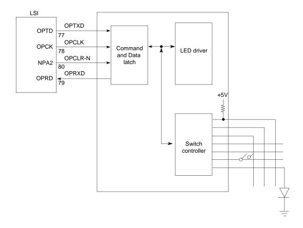
A 2-byte (15 bits + 1 even parity bit) command signal (OPTXD) is transmitted to the LSI (BU5148S) in synchronization with the OPCLK signal. The LSI decodes this command and when it is found to be legal, returns a 2-byte command response back to the LSI which includes data on Switch information, LED status, receive command ACK/NAK and 1 odd parity bit.
