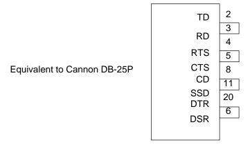
Figure C-3-6 Test Connector Connection Diagram
