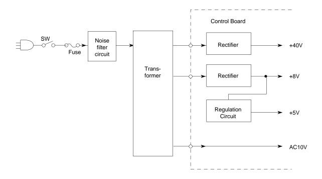
The uses of output voltages and signals are described below.
