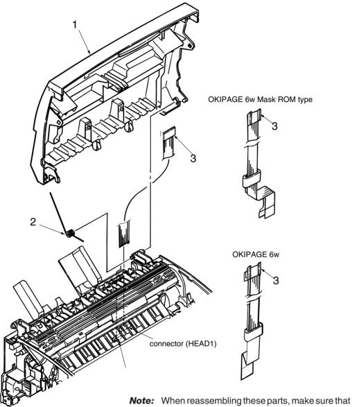
e: When reassembling these parts, make sure that the flat cable assy is firmly fitted with both the LED Head and connector Head 1 and Head 2. An improper fit may damage the control board and LED head.
