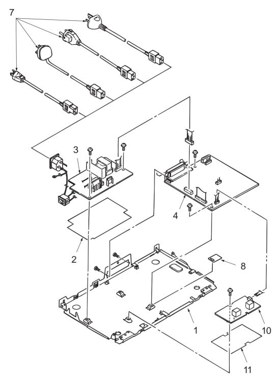
Figure 8-3-3 Base Plate Unit (OKIPAGE 6w Mask CPU type)
