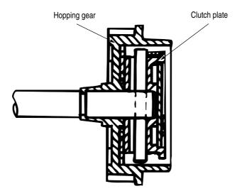
When the clutch is on, the hopping gear engages with the clutch plate to rotate the hopping roller.
