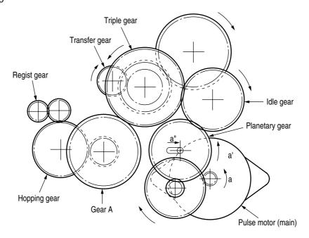
Rotate the pulse motor (main) in the a direction. The planetary gear rotates in the a' direction, dislocating its position in the a' direction. This causes the planetary gear to be separated from gear A. The hopping gear will not rotate. The triple gear and transfer gear rotate via the idle gear to drive the EP unit.
