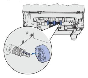
4. Push the pick roller onto the arm with the tab aligned. Repeat this step on the other side to install the other pick roller.
