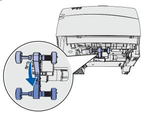
Press on the end of the tab and pull the pick roller off the arm. Repeat this step for the pick roller on the other side. Next, gently release the pick roller arm. Discard the used pick rollers. Remove the new pick rollers from their packaging.
