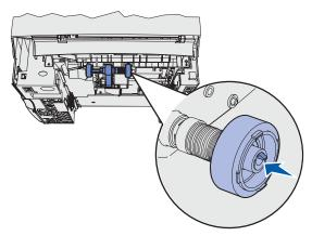
5. Gently release the pick roller arm. Insert the standard tray.
