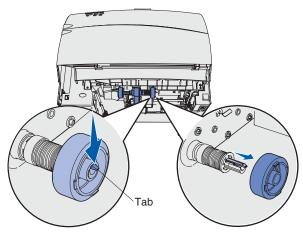
3. Pull the pick roller arm down. Locate the recessed area on the pick roller and align it with the tab on the arm. There are two arrows on each pick roller. Make sure the bottom arrow faces you as you align the recessed area with the tab.
